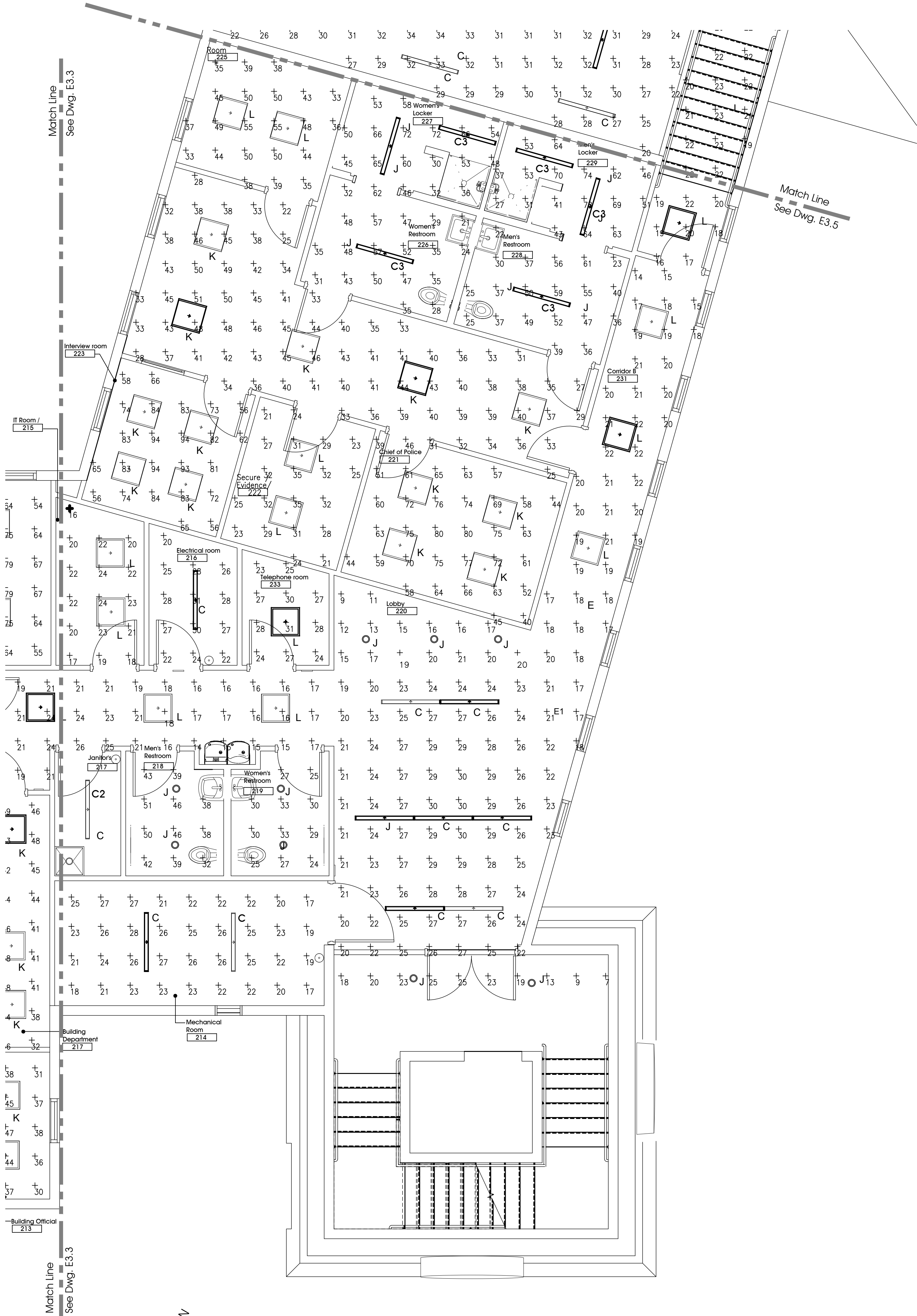
PARTIAL SECOND FLOOR PLAN PHOTOMETRICS (NORMAL LIGHTS) 1/4"=1'-0"
